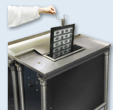
5. Seal image into aluminum
